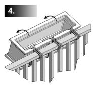
Hang the window box on the railing. Push the bracket extension tight against the hand rail and tighten the bolts with a wrench. Make sure all fasteners are firmly tightened.
