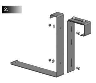
Align the deck rail bracket with the wall mount brackets that shipped with your Mayne window box. For the Yorkshire window box align the bottom 2 slots on the deck rail bracket with the Yorkshire wall mount bracket. Fasten them together using the 1/4 Hex Bolt, 1/4 Washer, and 1/4 nut. Tighten firmly with a wrench.
