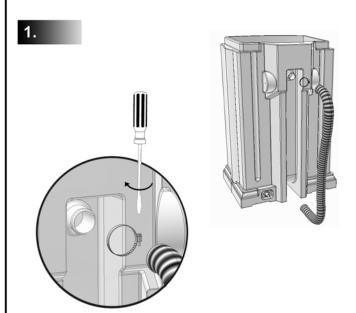
Attach the overflow hose (part 3) to the rain barrel overflow connector using the large clamp (part 6) to secure the hose in place. Tighten clamp with a slotted screw driver.
