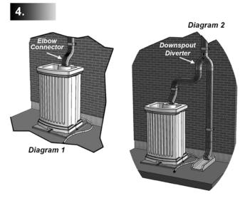
To complete the installation we recommend attaching an elbow to the end of the downspout (see diagram 1). A second option is the use of downspout diverter which has a lever to direct water into the barrel. Once the barrel is full you manually flip the lever back to direct water down the regular downspout (see diagram 2).
