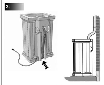
When placing your barrel under the downspout check that the ground is level and be sure to insert the overflow hose into the center channel as indicated by the arrow. We recommend using a patio stone to create a flat surface. Slightly angle the patio stone away from the house to direct run off water away from the foundation.
