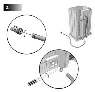
Attach the shut-off valve (part 7) to the threaded end of the garden hose (part 4). Next, attach the garden hose (part 4) to the rain barrel drain connector using the small clamp (part 5) to secure the hose in place. Tighten clamp with a slotted screw driver.
