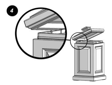
Snap fit lid design for secure fit.
