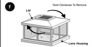
Remove the solar cap lid by holding the lens housing in place and then twist the lid in a clockwise direction. Be careful when twisting the lid to avoid damaging the tabs.
