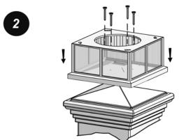
Place the lens housing on top of the post. Secure 4 screws through the holes in the solar cap adaptor plate (access through the circular hole in the lens housing).
