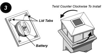
Be sure to pull the plastic tab from bottom of the lid to activate the battery (also check for correct orientation of the battery). Next, line up the lid tabs with the slots in the lens housing and twist counter clockwise to lock it in place.
