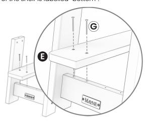
Add the second shelf (part E) and secure it with 4 - M5x45mm wood screws (part G).
