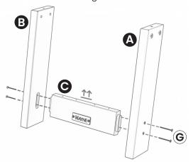
With 2 - M5x45mm wood screws (part G), attach one shelf (part E) to the first leg assembly. Align the pre-drilled holes as shown ensuring the counter sunk feature is facing upward. Underside of the shelf is labelled "bottom".
